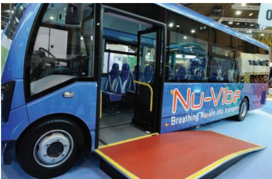
Nu-Vibe, from Nu-Track in Northern Ireland, employs Wright Group's Aluminique all-alloy body with quick-release panels
